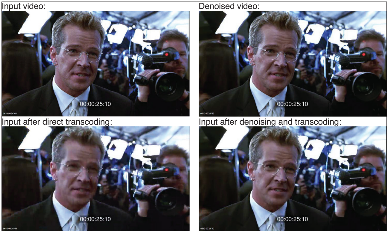
FIGURE 6. Example of using denoising filter for improving quality of the final transcoded signal.
