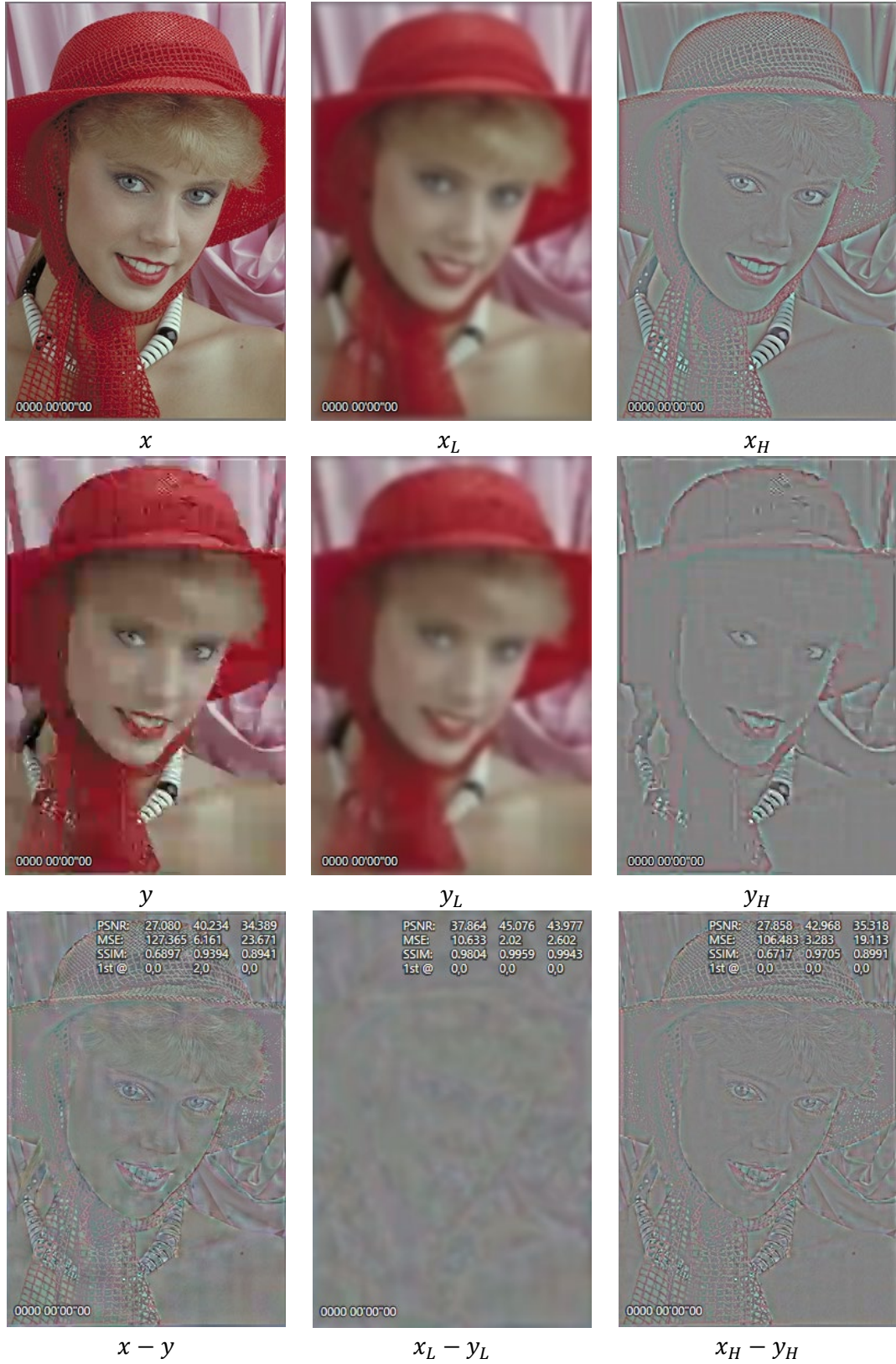
Fig. 2. Visual illustration of steps in the proposed model for computation of SSIM. The top row shows an input image x and its low-pass x_L and high-pass x_H = x - x_L versions. The middle row shows the second input image y , and its low-pass y_L and high-pass y_H = y - y_L versions. This image is an encoded and decoded version of x , with significant distortions introduced by the codec. The bottom row shows the differences between the original images, as well as their filtered versions. It can be observed that full difference is much “busier” and less descriptive than low- and high-pass differences. Low-pass emphasizes changes in overall shapes, while high-pass emphasizes changes in textures, contours, and other fine features.
